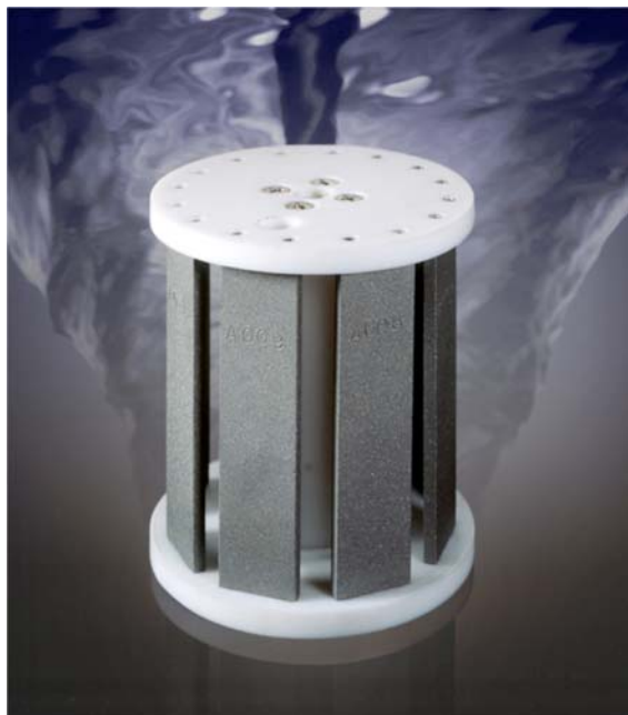
FIG. 2 Photo of Rotating Cage Containing Coupons
